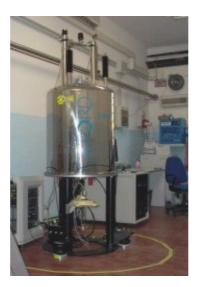
Model Gemini, 300 MHz, equipped with an Oxford 7 Tesla magnet and inverse and direct probe multinuclear. 1H, 13C e 31P mono- and bi-dimensional experiments are carried out both at room and at variable temperature.
