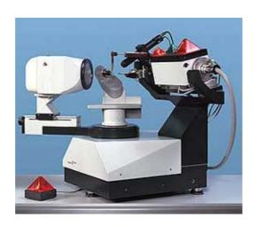
**Powder X-ray diffractometer Bruker D8 Advance:** XRD setting for structure analysis of polycrystalline and amorphous materials. Copper target X-ray tube used with curved-graphite monochromator. It is equipped with Ground Incidence Diffraction (GID) attachment.
